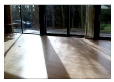
The South-facing orientation of the building making optimum use of natural light and 'passive solar gain' (i.e. by using the warmth of the sun to help with heating). The stone-filled gabions at the back of the hall help to store heat
